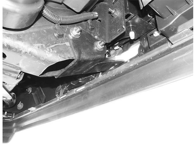
Driver/left side Frame Bracket installed
